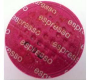
Foil imprint and poor perforation from a compatible capsule
